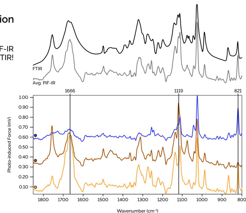
FIGURE 11. Similar to polarized FTIR, PiF-IR spectra are orientation sensitive due to the tip-enhanced field. The PiF-IR spectra above were acquired at different crystal faces on a vitamin C sample. They exhibit the local IR bands associated with the specific crystal faces. The average of these three distinct local PiF-IR spectra compare nicely with the bulk FTIR spectrum, which is the equivalent of an ensemble average of billions of PiF-IR spectra. Scan dimensions: 640 nm × 640 nm × 1025 nm.
